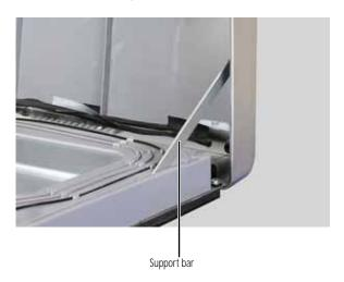
7 To close the case, make sure that all components, wires, and cables have been returned to their correct locations, then slowly close the panel while making sure no wires become pinched under the panel edges.
